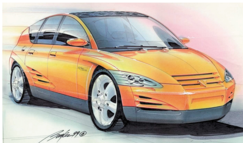
The aXcessaustralia car. The drive motor and transmission are at the front. In the rear is the internal combustion engine surrounded by the supercapacitor pack. The battery pack is located underneath the rear seats. Photo courtesy of CSIRO, Australia.
